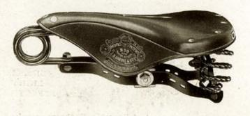
The model here illustrated has the usual pillar coil springs, and is the most resilient Saddle of that type.
