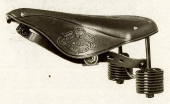
This model is designed on the same lines as our well-known B 104 but is of lighter build, and eminently suitable for light-weight Motor Cycles. In its construction are embodied the BROOKS Patent Compound Springs as described and illustrated on pages 6 and 7 of this List. The materials throughout are of the finest quality, and the leather top is most carefully and perfectly
